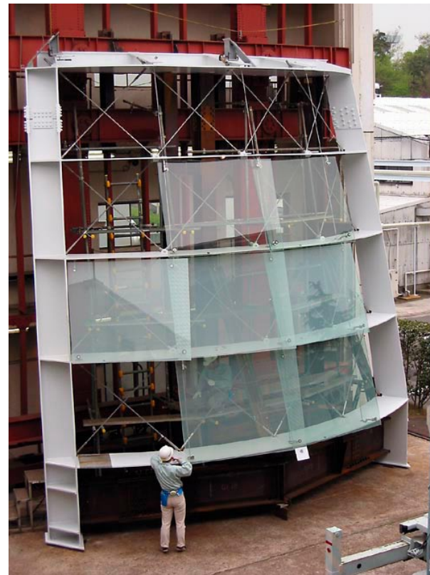
Figure 12 Buckled ring plate – applied three times heavier design force
